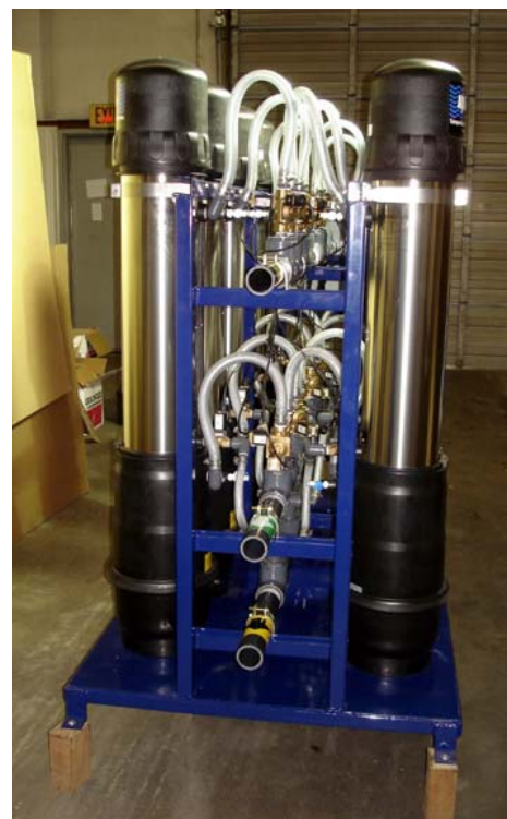
Example of a Portable Water Treatment System
